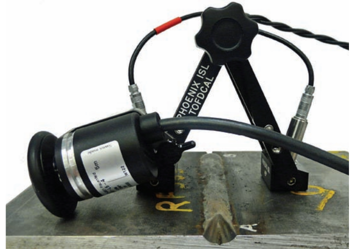
TOFD Caliper inspecting weld
